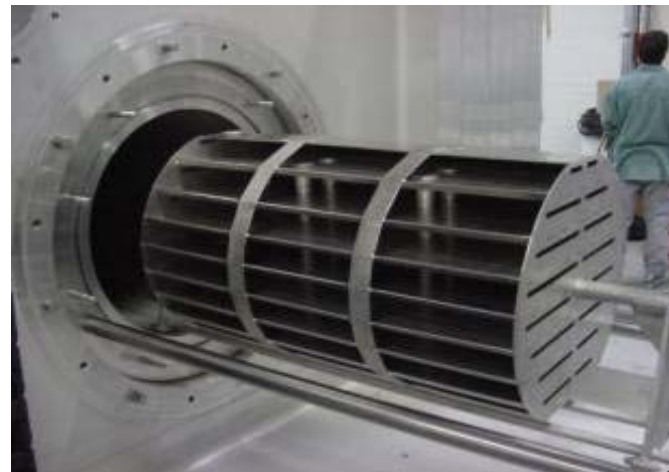
Drying calcination furnace
